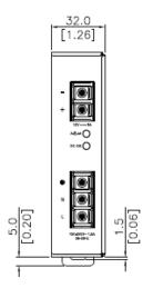
• 12 VDC Power Supply used to power the monitor
